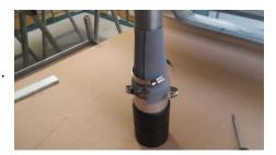
Turn the rudder to one side, and see the gaiter works well, Do the same to the other side.
