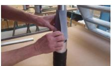
Open the clamps and put them around the stock. First tighten the lower one around the tube. Then press the top of the gaiter 30-50mm down, so it folds. Tighten the top clamp around the stock.
